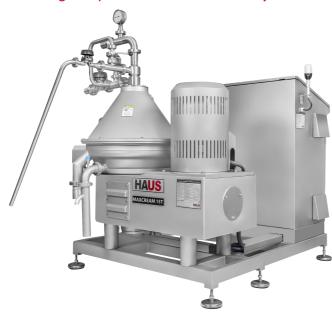
**THE PRODUCT** MAXCREAM 15T is a centrifugal separator configured as a concentrator for dairy application, with double paring discs, partial and total automatic discharge capabilities, and ready for Clean-In-Place (CIP).
